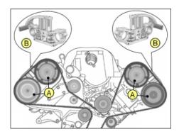
Do not replace complete camshaft adjusters (A) or camshaft adjustment housings (B).
